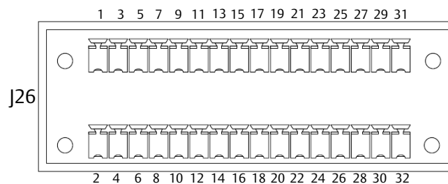
Figure 3-8 Dry contact port J26
