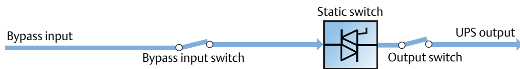
Figure 1-5 Schematic diagram of bypass mode
