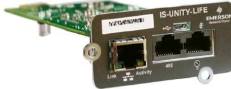
Figure 8-4 Appearance of IS-UNITY-LIFE card
