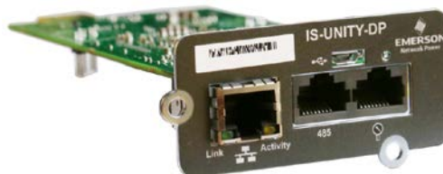
Figure 8-3 Appearance of IS-UNITY-DP card
